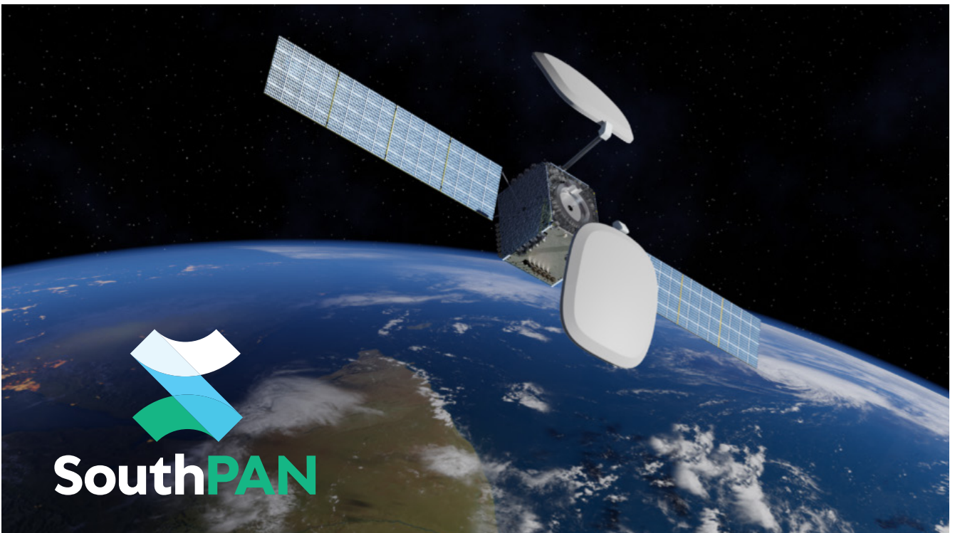
Artist's impression of an Inmarsat I-8 satellite, based on the SWISSto12 HummingSat platform.
