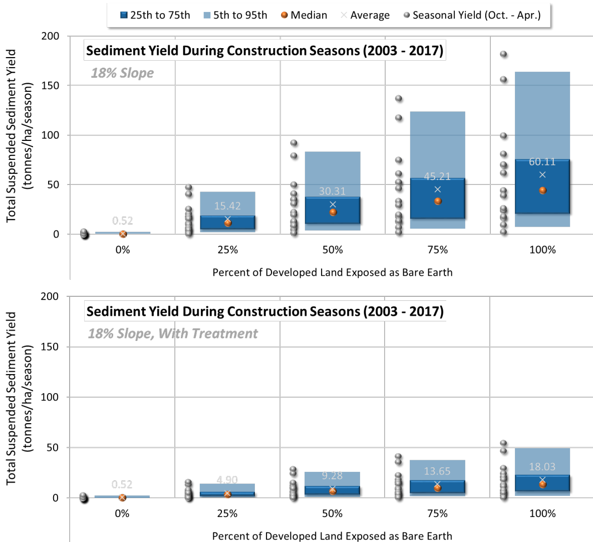
Figure 4: Simulated Effect of Staging on Sediment Yields for 18% Slope, with and without treatment.
